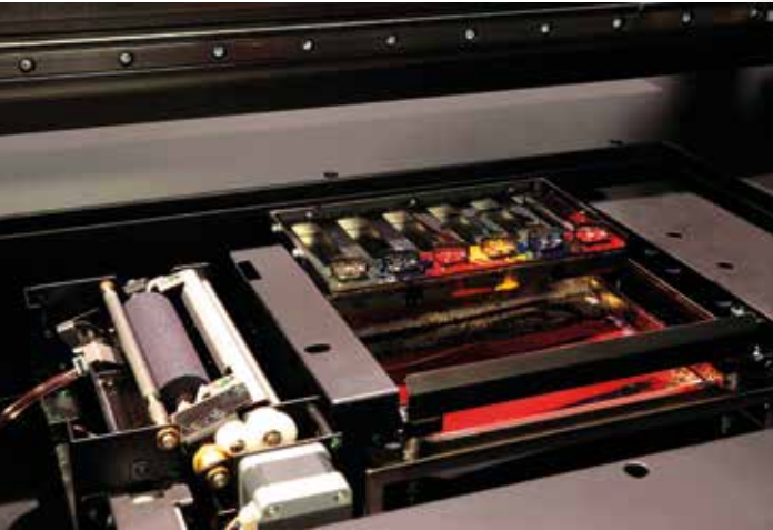
Automatic cleaning of print heads
