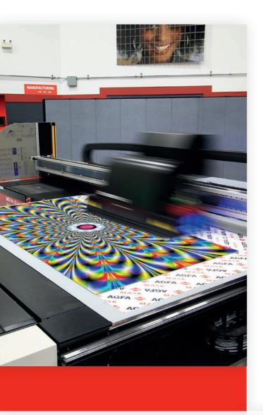
This award-winning flatbed printer now relies on UV LED curing to offer you impressive print quality on a wide variety of media. Accelerate the printing process to 248  $\mbox{m}^2/\mbox{h}$ , use the dockable roll-to-roll extension or opt for 3D Lens Technology printing whenever you need to.
